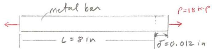
$$E = \frac{PL}{\delta A} = \frac{18 \text{ kip} (8 \text{ in})}{1.2 \text{ in.}^2 (0.012 \text{ in.})} = 10,000 \text{ ksi}$$
